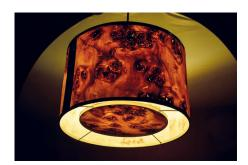
The **Orlina Pendant Light** was part of a lighting project that looked to utilise properties of wooden veneer as an alternative to solid timber. The Poplar Burr veneer was formed by soaking it in a solution containing a mix of different ingredients including Cascamite. This made the veneer less brittle and helped the veneer keep its organic form. The brass detailing that can be seen on the outside provides a crisp silhouette that covers the shadow of the overlapping veneers beneath.
