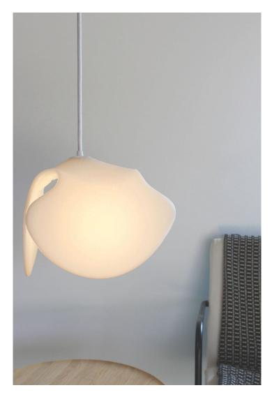
**Overlay** is a silicone pendant light that's unique shape is formed due to gravity and the flexibility of the material. The silicone is cast flat and when hung over the lamp holder it folds down into shape. This eliminates the need for a complex and expensive mould.
