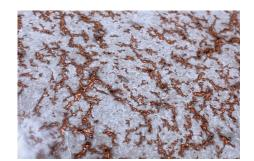
Remnant is a coffee table of an experimental nature which investigated the development and manipulation of paper and printing waste for the production of luxury furniture. The surface material, E-36, is a composite created almost entirely from the company's paper waste with a metallic grain. The surface's design is heavily inspired by Cubism, constructed using parquetry. The legs mirror this and are sealed in a thin coat of resin to protect the surface's texture.
